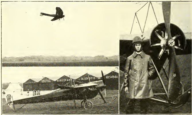
Three views of the reconstructed Handley Page monoplane (50 h.p. Gnome). In the right photograph is Mr. Whitehouse, who is now flying for Handley Page, Ltd. This machine now has ailerons for lateral control.
